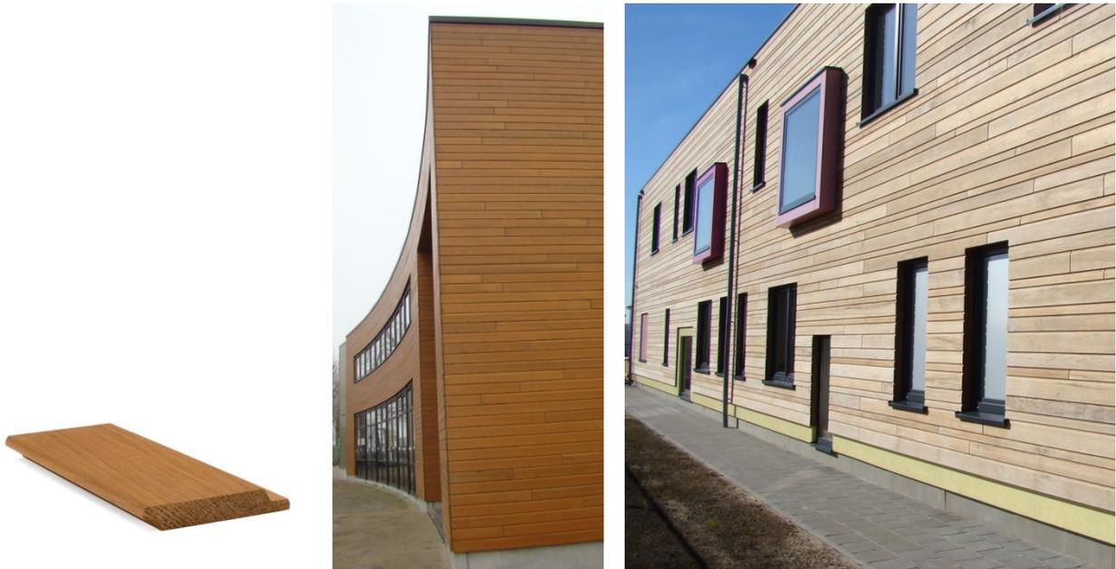
**Fig 1.5.** An example of thermally modified *T. superba* boards by Plato® (left) and two applications of cladding in the Netherlands (copyright: Plato®hout).
