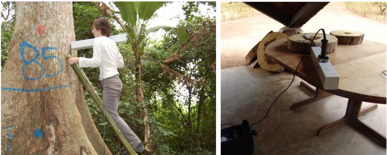
**Fig 6.2.** Drilling resistance measurements: in the field (left) and on freshly cut stem disks (right).
